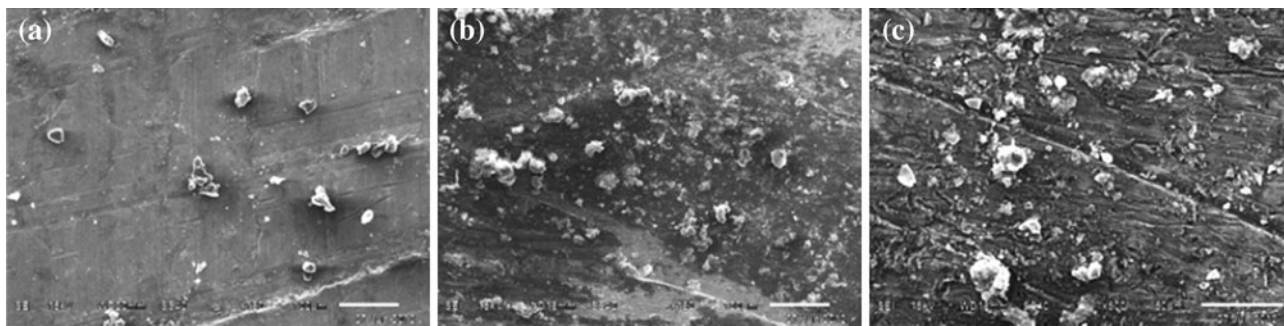
Fig. 1 Distribution of SiC p in ZC63 alloy matrix a 25 μm in size and 5 % in volume fraction, b 50 μm in size and 10 % in volume fraction, c 75 μm in size and 15 % in volume fraction
