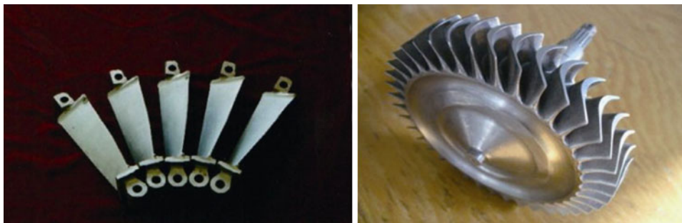
Fig. 6 Numerical controlled electrochemical machining of engine blades and integral impeller
