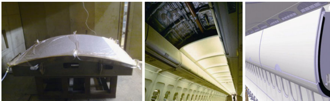
Fig. 5 Application of plant fiber composite on aircraft
