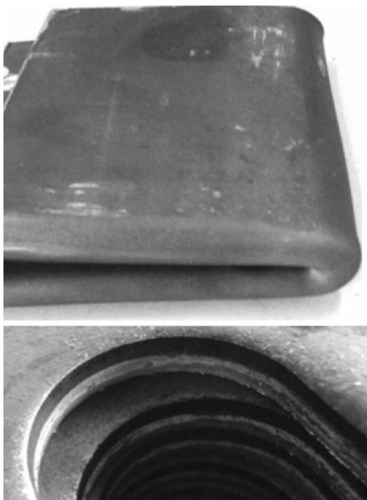
Fig. 13 Processing properties of 0.04 %C-1.4%Mn-0.09 %Nb steel with regard to bendability and hole punching
