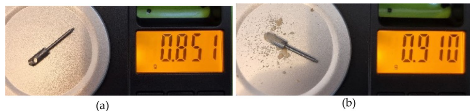
Fig. 3 (a) BKS, innovative biomechanism for bone screws and implants dry weight before insertion into the bones; (b) and BKS filled with synthetic bone after application MRT, showing total weight after removal from bone
