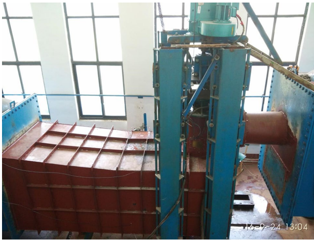
Fig. 8 Picture of the non-full passage model pumping system installed on test bench
