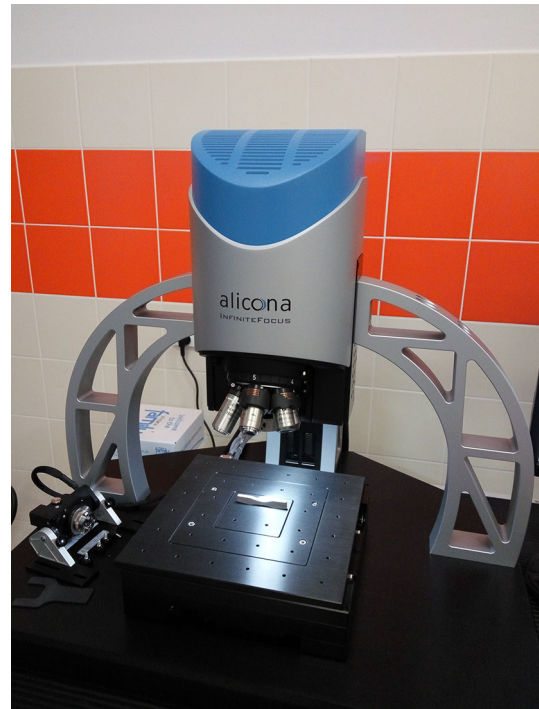
Fig. 2 Focus variation microscope InfiniteFocus® IF G5 used in the experimental investigations
