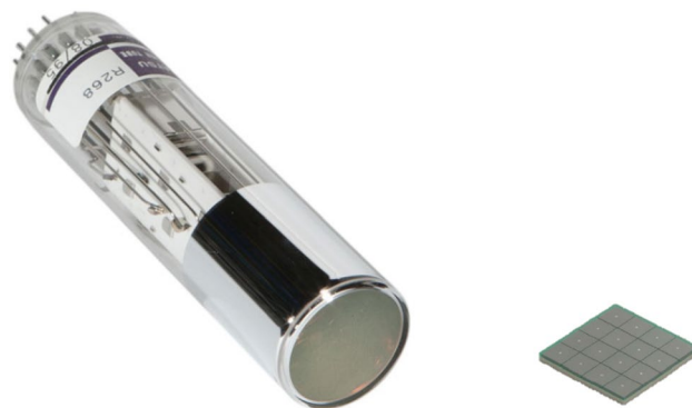
Fig. 1 Photomultiplier tube (PMT) (left) and silicon photomultiplier (SiPM) (right)
