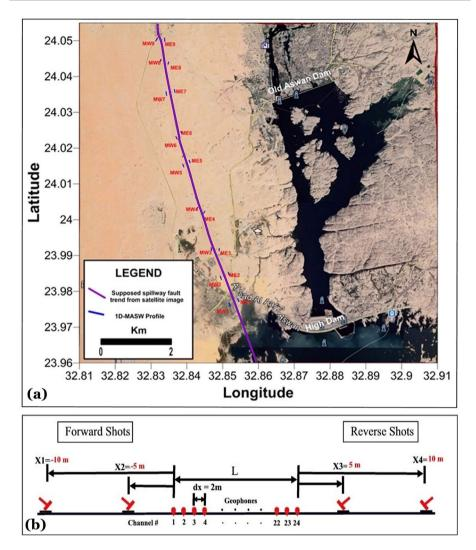
Fig. 14 Location map of the seismic MASW profiles around supposed Spillway fault (a), the Source-Receiver configuration with a standard fixed roll along for 1D MASW field survey (b)
