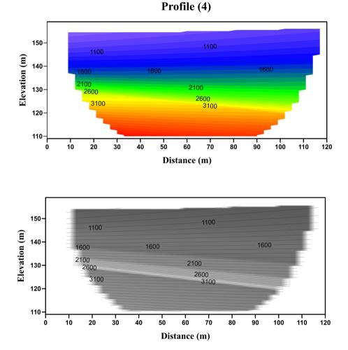
Fig.8 Seismic velocity section along profile No.4 (Up) The 2-D velocity section, and (Down) Structural section (the P-wave velocity in m/s)
