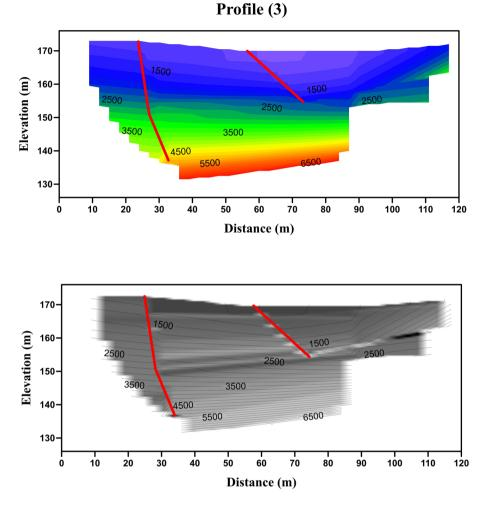
**Fig. 7** Seismic velocity section along profile No.3. (Up) The 2-D velocity section, and (Down) Structural section (the P-wave velocity in m/s and the red line represents fault)
