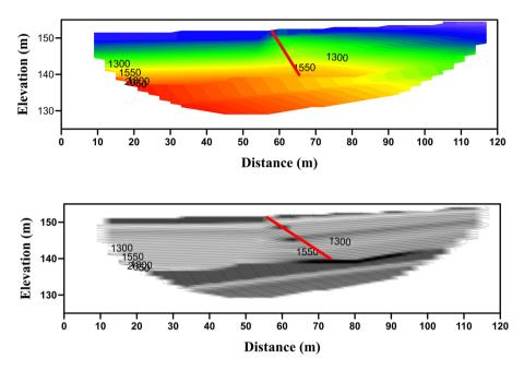
Fig. 9 Seismic velocity section along profile No.5 (Up) The 2-D velocity section, and (Down) Structural section (the P-wave velocity in m/s and the red line represents fault)
