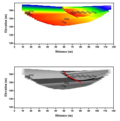
Fig. 11 Seismic velocity section along profile No.7 (Up) The 2-D velocity section, and (Down) Structural section (the P-wave velocity in m/s and the red line represents fault)
