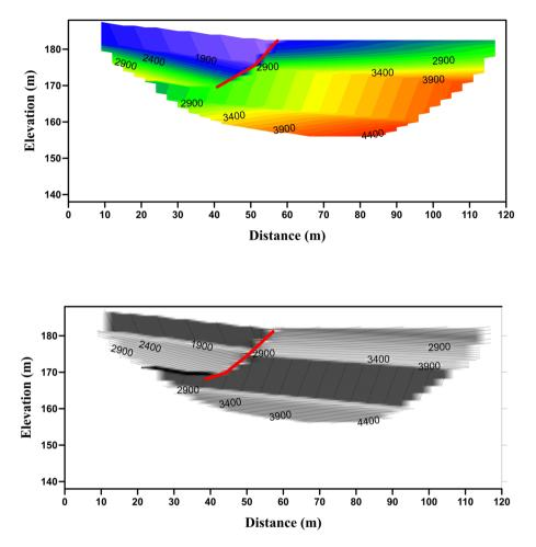
Fig. 12 Seismic velocity section along profile No.8(Up) The 2-D velocity section, and (Down) Structural section (the P-wave velocity in m/s and the red line represents fault)
