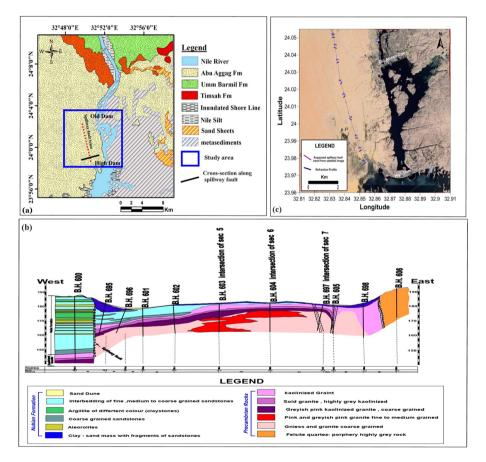
**Fig. 2** Geological map of the Aswan High Dam area (after EGSMA 2002) (**a**), cross-section along spillway fault (WCC,1985) (**b**), and the location map for the seismic refraction profiles along the Supposed spillway fault trace (**c**)
