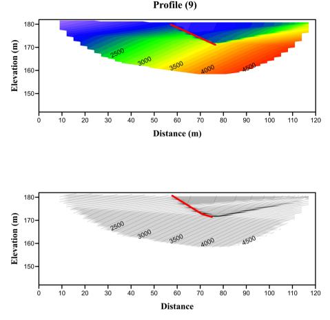
**Fig.13** Seismic velocity section along profile No.9 (Up) The 2-D velocity section, and (Down) Structural section (the P-wave velocity in m/s and the red line represents fault)
