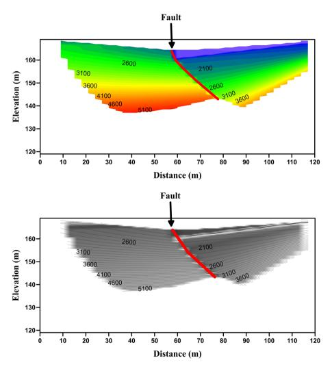
**Fig. 10** Seismic velocity section along profile No.6 (Up) The 2-D velocity section, and (Down) Structural section (the P-wave velocity in m/s and the red line represents fault)
