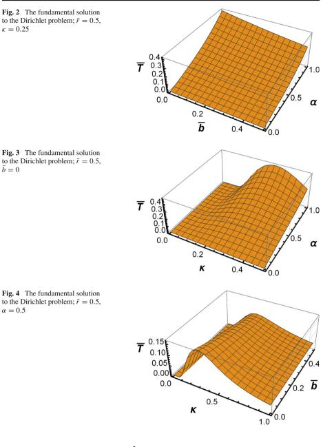
$$\frac{\partial^{\alpha} T(r,t)}{\partial t^{\alpha}} = a \left[ \frac{\partial^2 T(r,t)}{\partial r^2} + \frac{2}{r} \frac{\partial T(r,t)}{\partial r} \right] - bT(r,t),$$
