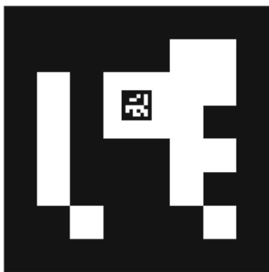
Fig. 6 Modified ArUco marker. An smaller marker is placed in a bigger one.
