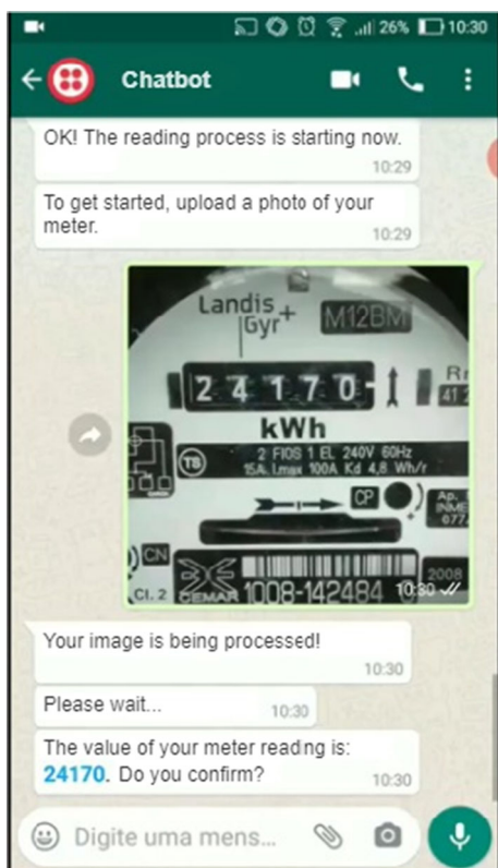
Fig. 12 The chatbot solution presenting in the chatting app the self-reading result from an image sent by the consumer
