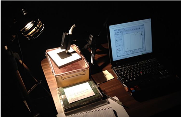
Fig. 10 ASD Spectrometer set-up with material placed on a Spectralon panel, quartz lamp, and pistol fiber feed to spectrometer/computer. The set-up shows an approximate 90-degree phase angle from illumination source-target-detector
