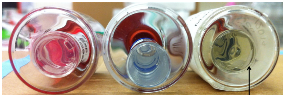
Fig. 1 Images of DMTS-PS80 water formulations prepared by each laboratory at the start of the stability study show some evidence of instability. Shown are representative samples from each of the three PS80 DMTS formulations prepared by each laboratory from a bottom view (B formulation, far left; A formulation, middle; C formulation,
