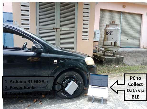
Fig. 23 Tire Strain Measuring Method
