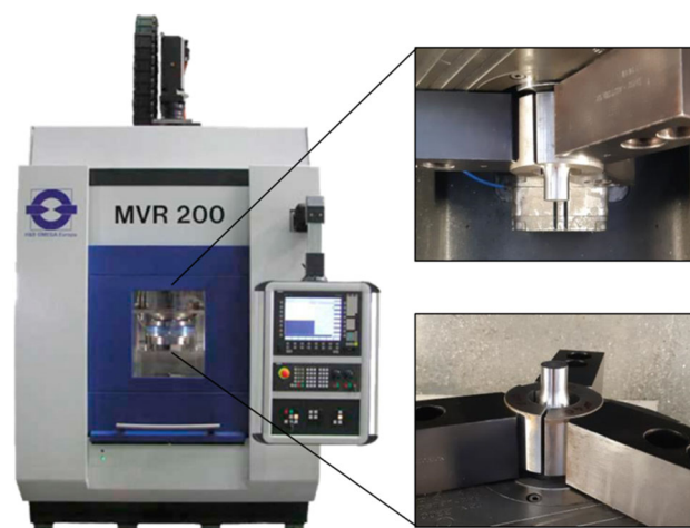
Fig. 4 Machine setup for welding the specimens
