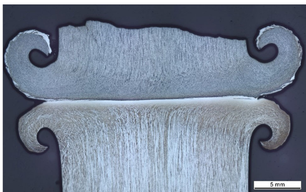
Fig. 11 Fatigue crack initiation at a specimen with flash under torsional loading starting from the surface of the base material
