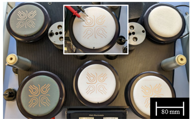
Fig. 3 Martindale instrument with fixed samples and how the conductivity is measured
