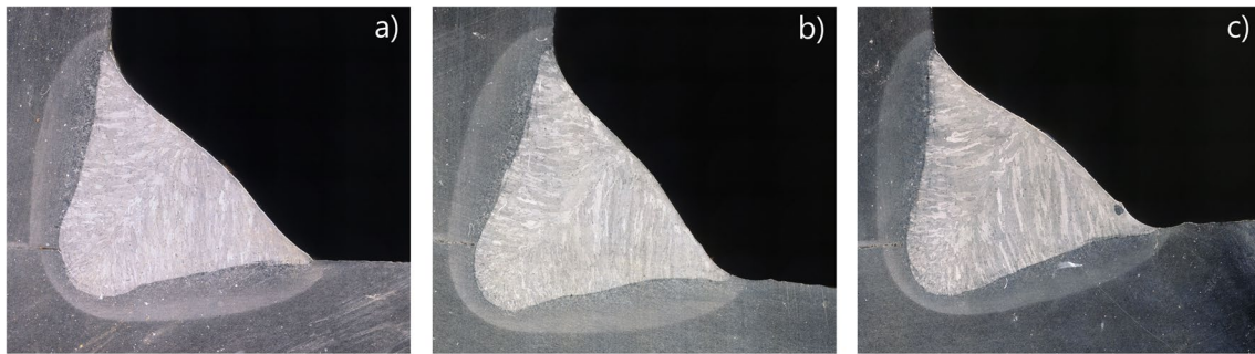
Fig. 10 Polished sections of an AW specimen (a), a manual HFMI-treated weld toe (b) and an automated HFMI-treated weld toe (c)
