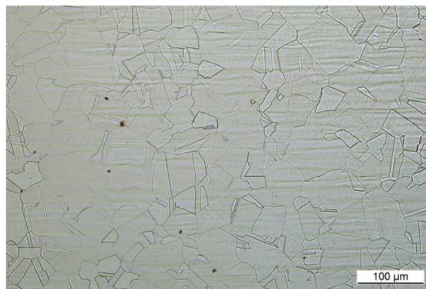
Fig. 1 Austenitic microstructure of the X2CrMnNi17-7-5 base material with obvious rolling structure
