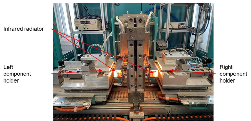
Fig. 1 Modified welding machine for radiation welding (bielomatik GmbH, Heraeus Noblelight GmbH)
