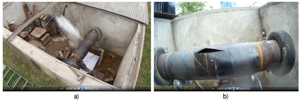
Fig. 11 The burst test of the FSPS3 DN300 pipe section: a end of the burst test (recorded from above); b the pipeline section after the test
