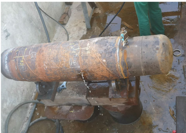
Fig. 14 The FSPS4 DN350 pipe section after the burst test
