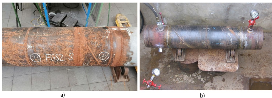
Fig. 6 Full-scale pipeline sections: a cut DN350 pipe with the two tested girth welds before the formation of the pipeline section FSPS4; b FSPS3 DN300 pipeline section before the beginning of the fatigue test
