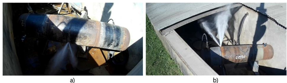
Fig. 15 a End of the burst test of the FSPS5 DN400 pipeline section (recorded from above); b end of the burst test of the FSPS6 DN400 pipeline section (recorded from above)
