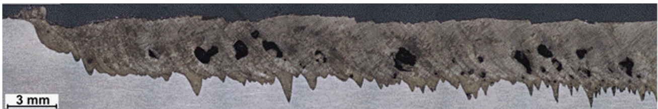
Fig. 9 Exemplary metallographic longitudinal-section of an aluminum sample welded with the combination of 3.1 kW TruDisk12002 and 0.6 kW YLR-1000SM for the focal plane F_{YLR} = -2 mm
