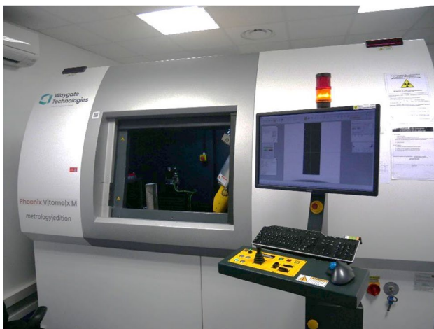
Fig. 12 Waygate Technologies vltomelx m 300/180 XCT from Baker Hughes used to inspect the investigated parts
