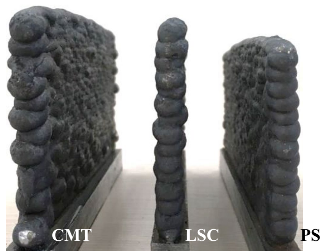
Fig. 1 General view of deposits manufactured using the different deposition modes: CMT, LSC and PS
