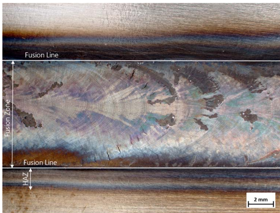
Fig. 2 Illustration of different regions and boundaries that were used in the crack evaluation of UNS S31035 base material
