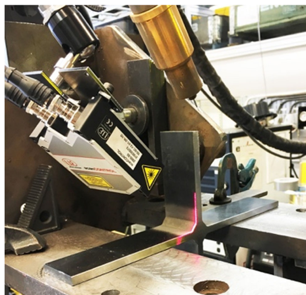
Fig. 4 Laser setup for geometry evaluation
