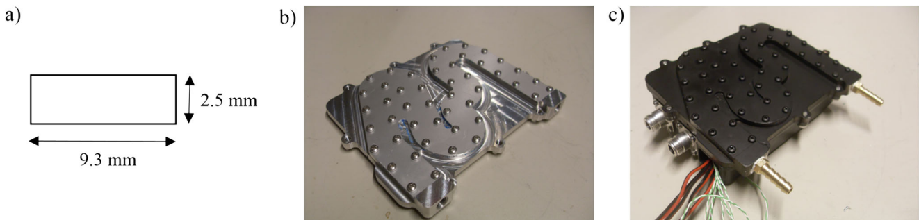
Fig. 6 The prototype with the milled a rectangular channel having dimension of 2.5 \text{ mm} \times 9.3 \text{ mm} , b the prototype after sealing the channel with a screwed lid, and c the assembled prototype
