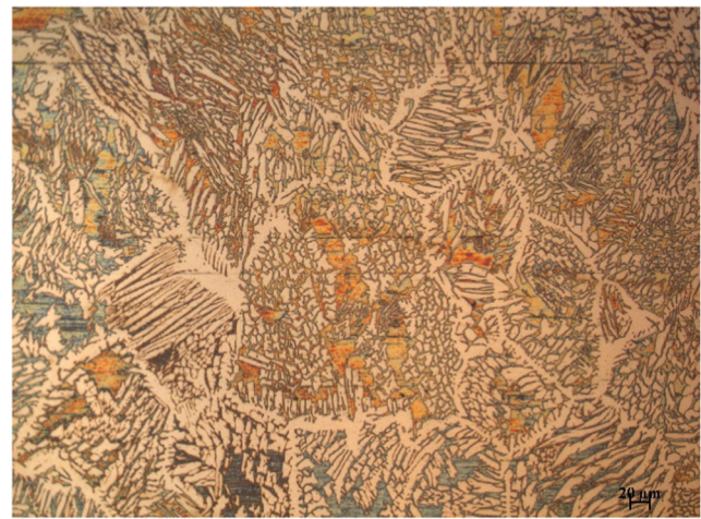
Fig. 3 LOM micrograph of alloy 4: [F] solidification mode showing Widmanstätten austenite plates in the former ferrite grain boundaries and formed in the solid phase after solidification. Austenite is revealed in white colour whilst ferrite is shown in blue and yellow. Ferrofluid EMG 911 was the etching solution
