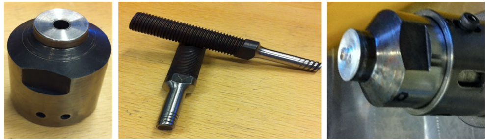
Fig. 3 The friction stir welding tool: a shoulder (smooth with 3.6° concavity and 17-mm diameter); b probe (conical with LH threads of 1.5-mm pitch); c shoulder and probe assembled in tool body
