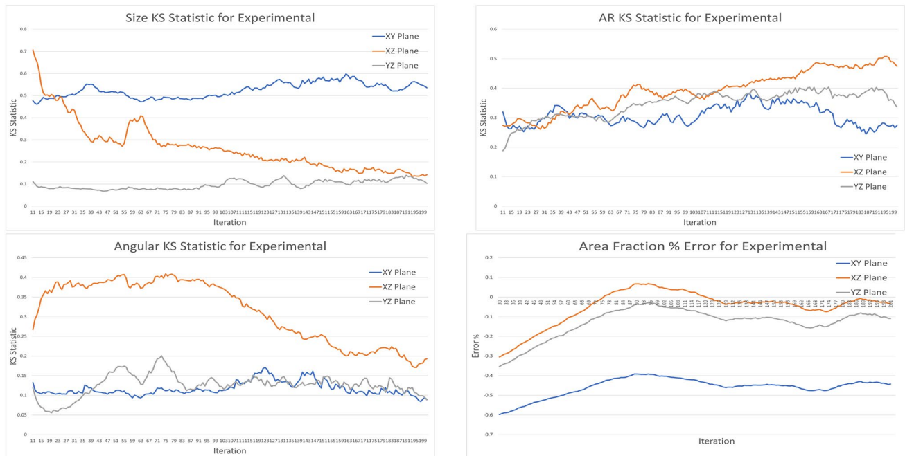
Fig. 12 M_a of the size, shape, and 2D angle distribution KS test statistics and area fraction percent error progression of the experimental data. Moving average is calculated based on 10 observations at time;
