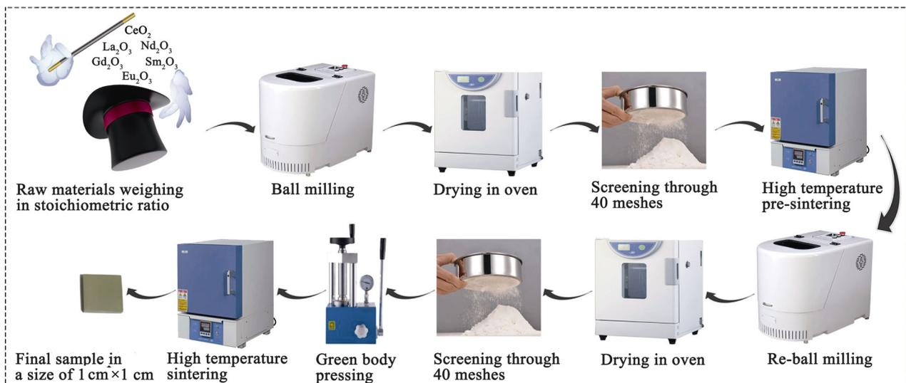
Fig. 1 Preparation process of high-entropy  $(\text{La}_{0.2}\text{Nd}_{0.2}\text{Sm}_{0.2}\text{Eu}_{0.2}\text{Gd}_{0.2})_2\text{Ce}_2\text{O}_7$ .
