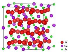
Fig. 1 Crystal structure of Gd<sub>2</sub>Zr<sub>2</sub>O<sub>7</sub>.
