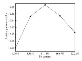
Fig. 3 Variations of lattice constant with the Sc content.
