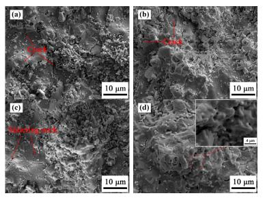
Fig. 10 Surface morphologies of Gd–Sc coatings after heat treatment at 1400 °C for (a) 20 h, (b) 50 h, (c) 100 h, and (d) 200 h.
