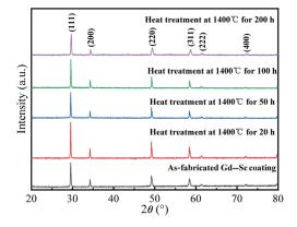
**Fig. 9** XRD patterns of Gd–Sc coatings after different heat treatment time.
