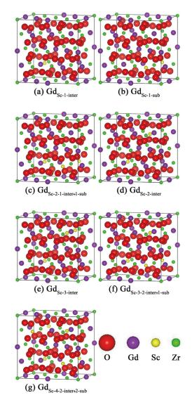
Fig. 2 Solid solution mode of Sc in  $Gd_2Zr_2O_7$  lattice with different doping contents.
