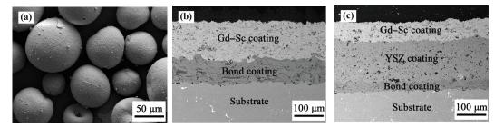
Fig. 8 (a) Surface morphology of Gd–Sc spraying powders, and cross-sectional microstructures of (b) Gd–Sc TBC and (c) Gd–Sc/YSZ DCL TBC.
