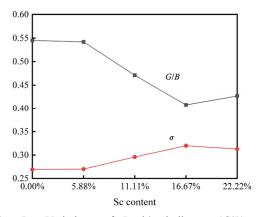
**Fig. 5** Variations of Pugh's indicator (*G*/*B*) and Poisson's ratio ( $\sigma$ ) with the Sc content.
