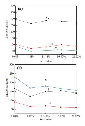
**Fig. 4** Variations of (a) elastic constants  $C_{11}$ ,  $C_{12}$ ,  $C_{44}$ , and (b) bulk modulus *B*, shear modulus *G*, and Young's modulus *E* with the Sc content.
