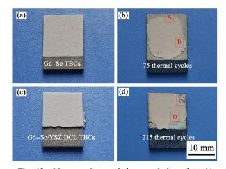
**Fig. 12** Macroscopic morphology evolution of (a, b) Gd–Sc TBCs and (c, d) Gd–Sc/YSZ DCL TBCs during thermal cycling tests.
