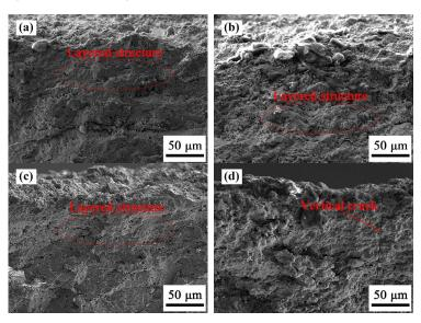
Fig. 11 Fracture surface morphologies of Gd–Sc coatings after heat treatment at 1400 °C for (a) 20 h, (b) 50 h, (c) 100 h, and (d) 200 h.
