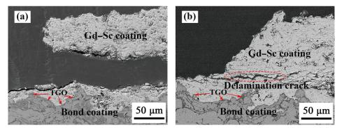
Fig. 14 Cross-sectional microstructures of regions (a) A and (b) B of Gd–Sc TBCs after 75 thermal cycles.
