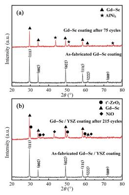
**Fig. 13** XRD patterns of (a) Gd–Sc TBCs and (b) Gd–Sc/YSZ DCL TBCs after thermal cycling tests.
