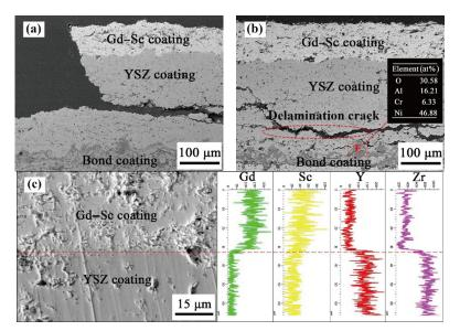
**Fig. 15** Cross-sectional microstructures of regions (a) C and (b) D of Gd–Sc/YSZ DCL TBCs after 215 thermal cycles. (c) EDS line scanning of the interface between Gd–Sc and YSZ coating.
