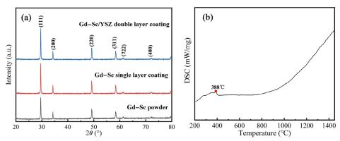
Fig. 7 (a) XRD patterns of Gd–Sc powders and coatings, and (b) DSC curve of Gd–Sc powders.
