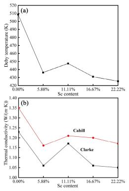
Fig. 6 Variation of (a) Debye temperature  $\Theta$  and (b) thermal conductivity with the Sc content.
