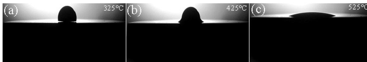
Fig. 6 Wettability measurements wherein contact angle was analyzed using ImageJ software: (a) carbonate pellet on the 50CP–50PSFC substrate, (b) incipient melting of carbonate pellet, and (c) spread carbonate drop.
