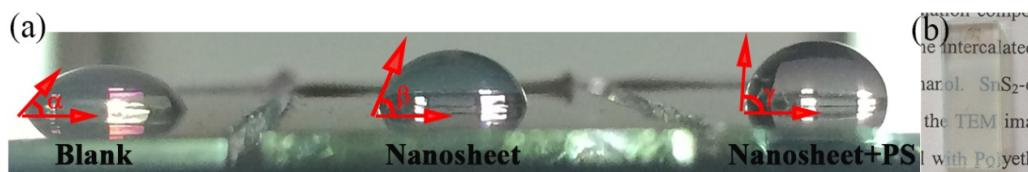
Fig. 5 (a) Infiltration angle measurements performed for blank glass, nanosheet-coated glass, and glass coated with nanosheets +3wt%PS ( \alpha=45^\circ , \beta=65^\circ , \gamma=90^\circ ); (b) the sensing film.
