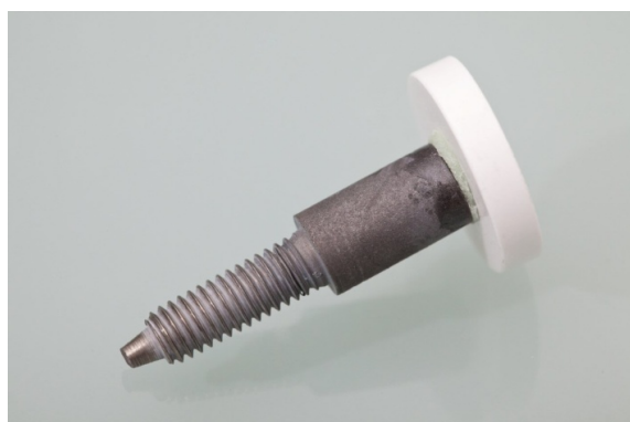
Fig. 1 Traction–adhesive strength test assembly with TiAlV probe (left side) cemented onto a ZPTA disc. For bonding between probe and disc, there is a thin layer of bone cement (Palacos ® , about 0.2 mm thick). The dark shading of the surface in the cylindrical area of the probe near the cement layer (opposite to the thread) is part of the protecting PolyMA coating unintentionally in excess applied to the front side of the probe.
