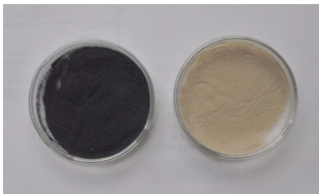
Fig. 1 The as-received coarse powders “C” (Metco 6232B) (left) and its thermally oxidized powders “COX” (right).
