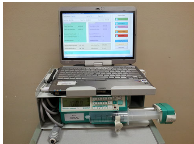
Fig. 3 The patient-controlled epidural analgesia system utilizing a Hewlett Packard Compaq Tablet PC connected to a modified B. Braun Perfusor R Compact S infusion pump
