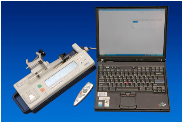
Fig. 1 First generation computer integrated infusion pump set-up using an IBM Thinkpad laptop (IBM, USA) connected to a modified infusion pump (IVAC P700, Alaris, UK)
