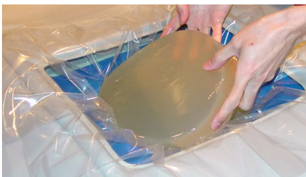
Fig. 5 The MRgFUS transducer assembly is mounted on a positioning system, all of which is sealed in a plastic chamber filled with de-gassed de-ionized water and installed in a specially designed MR compatible table. For fibroid treatments a gel pad is placed on top of the window in this plastic chamber, as depicted in this photograph. (Photograph, courtesy of Insightec Ltd.)
