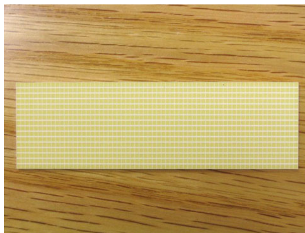
Fig. 3 A 64-slice scintillator array. The scintillator (yellowish material) is segmented by a reflector (white strips). The reflector’s primary function is to keep the light generated in a detector element within that element to minimize cross-talk (photo courtesy of Philips Healthcare) (Color figure online)
