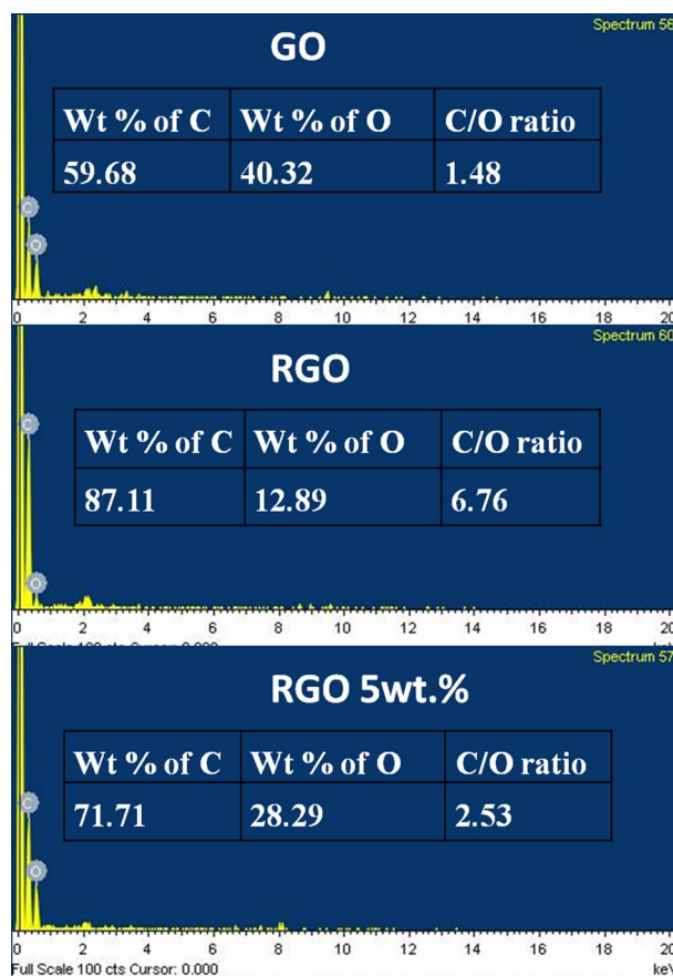
Fig. 5 EDS measurement of GO, RGO and RGO/GO hybrid (5%) and the corresponding C/O ratio
