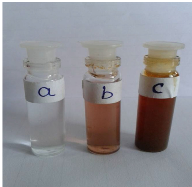
Fig. 1 a Aqueous solution of copper nitrate, b aqueous extract of tea leaf, c color of the solution after the reaction
