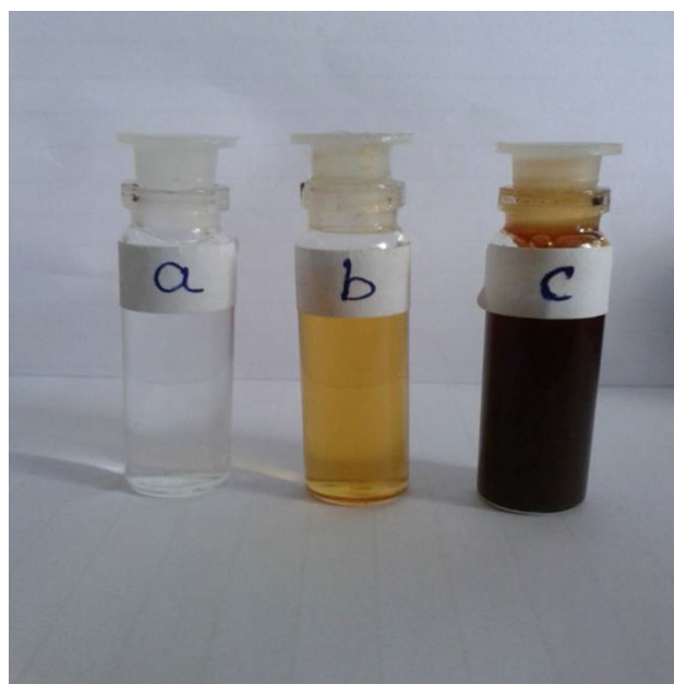
Fig. 5 a Aqueous solution of copper nitrate, b aqueous extract of coffee powder, c color of the solution after the reaction
