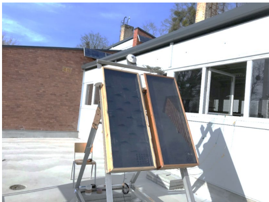
Fig. 4 Tested solar air collectors
