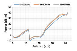
Fig. 5 Circuit output power versus axial distance in, V = 3200 v
