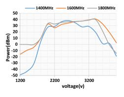
Fig. 4 Circuit output power versus of the electron beam voltages
