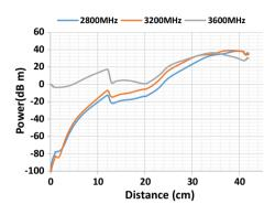
Fig. 6 Circuit output power versus axial distance, V = 3200 v
