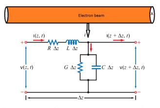
Fig. 1 Each section of the helix is represented by an equivalent circuit [16]
