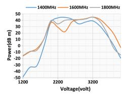
Fig. 2 Circuit output power versus of the electron beam voltages
