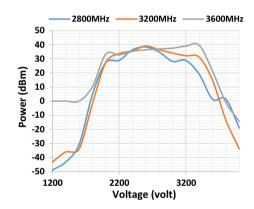
Fig. 7 Circuit output power versus beam voltage
