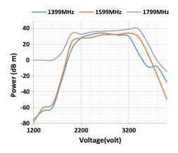
Fig. 8 Circuit output power versus beam voltage
