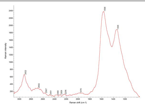
Fig. 4 Raman spectrum of CNT synthesized by CVD method
