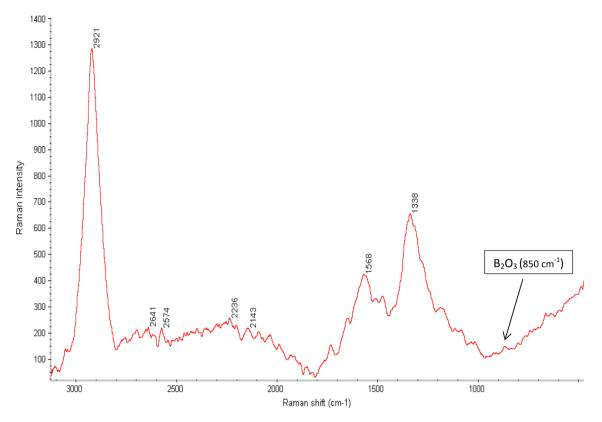
Fig. 5 Raman spectrum of CNT/B<sub>2</sub>O<sub>3</sub>
