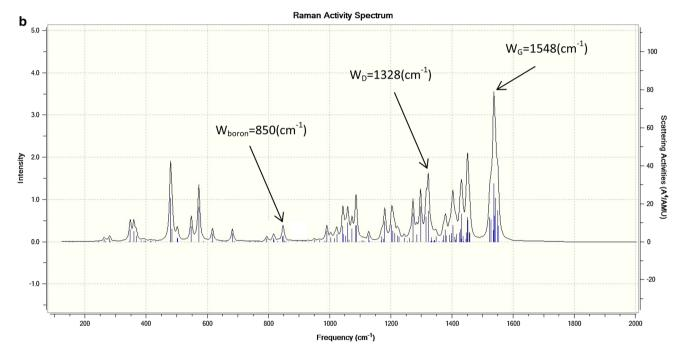
Fig. 9 a Schematic illustration of boron-doped CNT. b Theoretical calculation of Raman spectrum of boron-doped CNT
