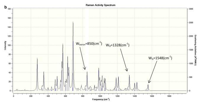
Fig. 10 a Schematic illustration of CNT/boron-Ag NPs. b Theoretical calculation of Raman spectrum of CNT/boron-Ag NPs
