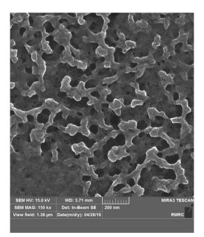
Fig. 1 SEM image of doped CNTs (CNT/B<sub>2</sub>O<sub>3</sub>)
