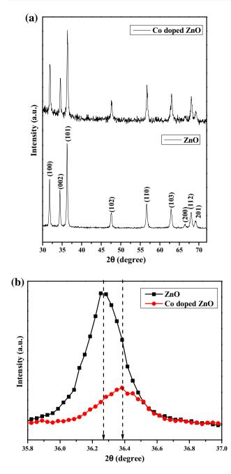
Fig. 1 X-ray powder diffraction pattern of (a) pure ZnO and Co doped ZnO NPs and (b) an enlarged version of the XRD pattern between  $35.8^\circ$  and  $37^\circ$
