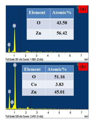
Fig. 3 EDAX spectra of (a) pure ZnO, and (b) Co doped ZnO NPs
