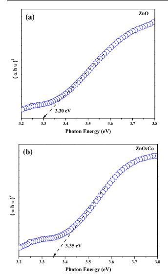
Fig. 5 Band gap measurement for n = 1 excitonic state of (a) ZnO NPs and (b) Co doped ZnO NPs
