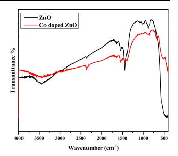
Fig. 4 FT-IR absorption spectra of (a) ZnO NPs and (b) Co doped ZnO NPs
