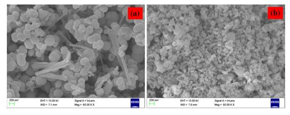
Fig. 2 FESEM image of (a) pure ZnO, and (b) Co doped ZnO NPs
