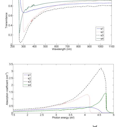
**Fig. 6** Absorption coefficient of carbon nanostructure suspensions in different liquids
