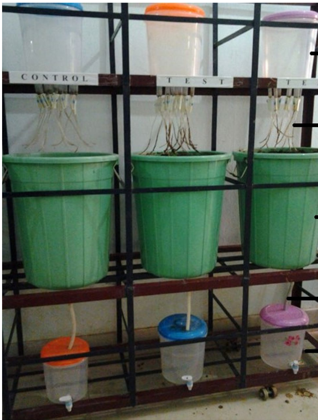
Fig. 3 Assembled vermifiltration unit
