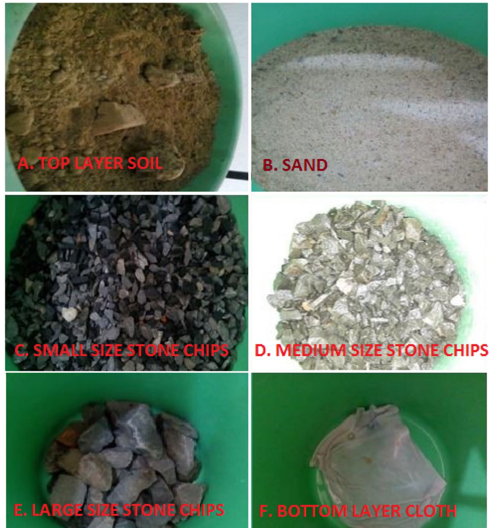
Fig. 5 Different layers of vermi-filter bed
