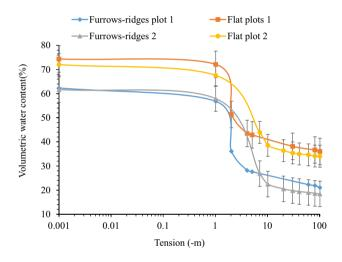
Fig. 2 Variation of soil water content as a function of production period and soil tillage mode
