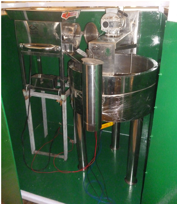
Fig 2 Prototype waste processing machine (inside view)
