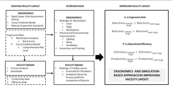
Fig. 1 Ergonomics and simulation-based approach in improving facility layout
