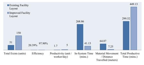
Fig. 4 Comparison of existing and redesigned facility layout
