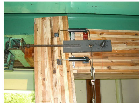
(b) Pullout failure of LSB in column
