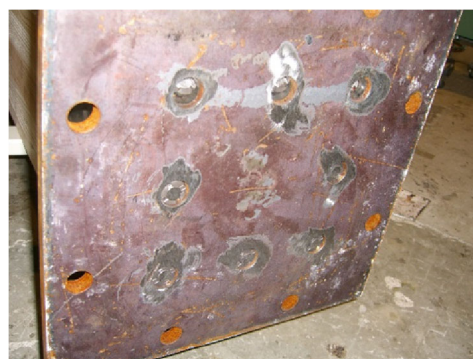
(c) Partial tensile failure of connection between LSB and column base joint
